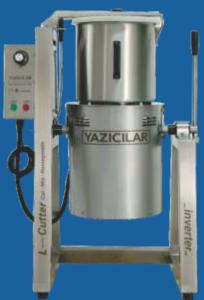
L20IV is the standing model with a 20 Liter bowl, variable speed and 230V connection L20I-Lab is the standing model with a 20 Liter bowl, variable speed and 380V connection
